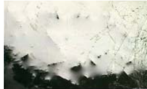
(2) Intermetallic crystals precipitate
